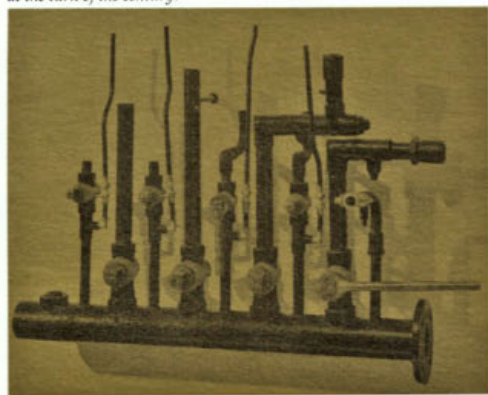
Early gas light mechanism, as was commonly used in both Canadian and American theatres at the turn of the century.
